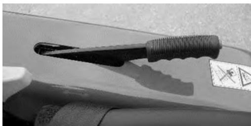
The parking brake is released in position "A"
