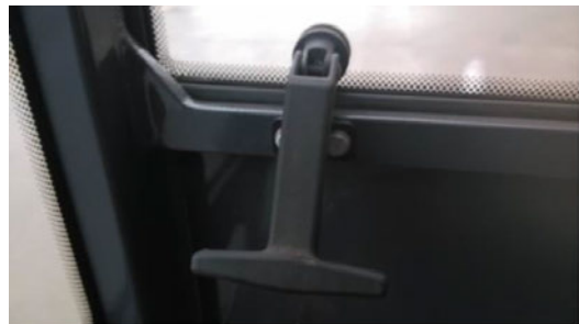
Pull both handles at the same time, to close the rear window
